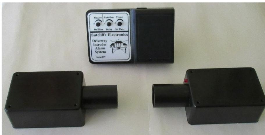
A Wired active Infrared beam device to give warning of the arrival of a visitor on your property, and which can also be used to trigger a warning siren or floodlights for your own convenience.
