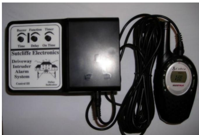
Part of the adaption is designed to give a maintenance charge to the internal battery set in the radio. Thus it can be left connected permanently.
