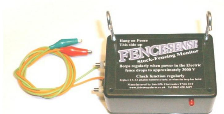
A device to give warning that your electric stock fence is not functioning correctly. Once the voltage in an electric fence has dropped to about 3000V or below, it is rapidly reaching the point when it is no longer effective. The FENCESENSE gives a regular loud beep when this point is reached, allowing the fault to be rectified before the animals get out.
