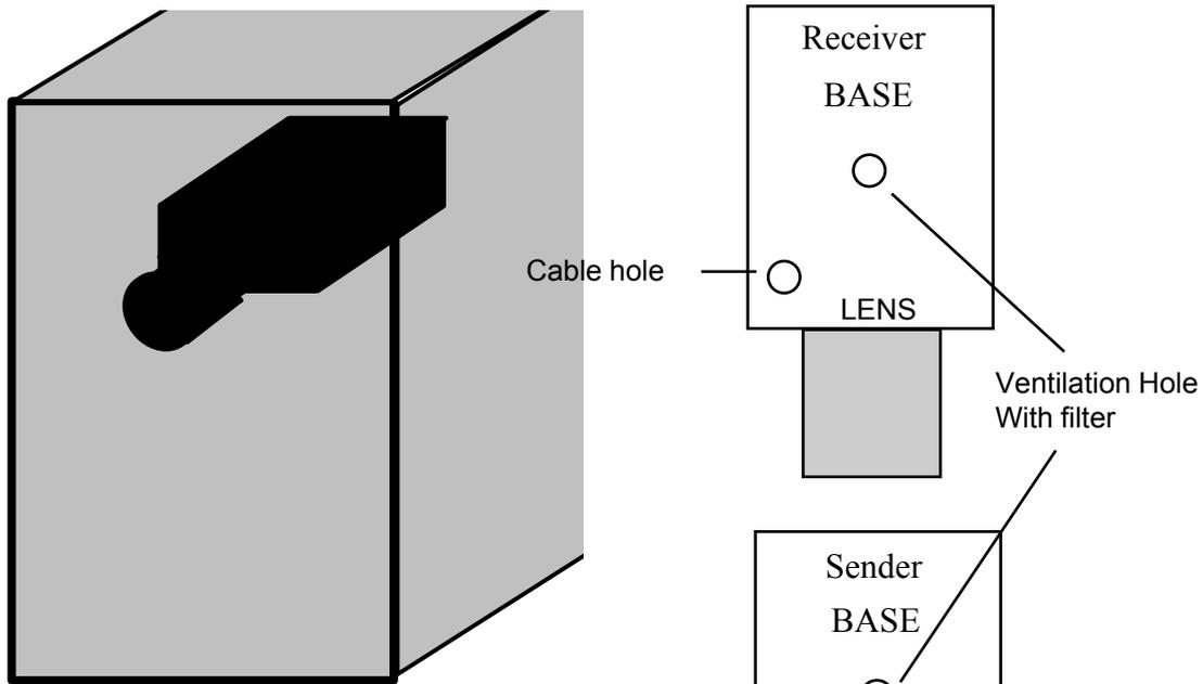
Mount the beam boxes inside rather than on a post. Hollow posts can be made from four planks nailed together
